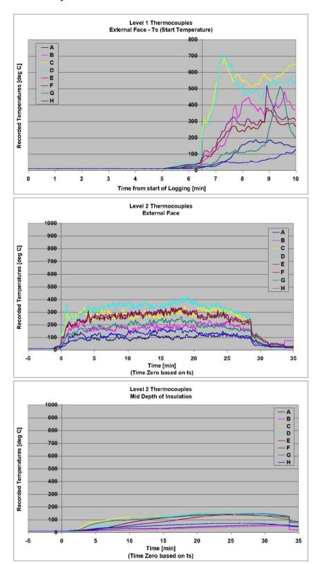
No Panel joint penetration - Test terminated 35:00
