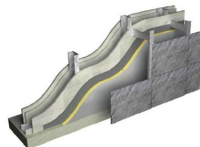
Celotex RS5000 in a rainscreen cladding application
