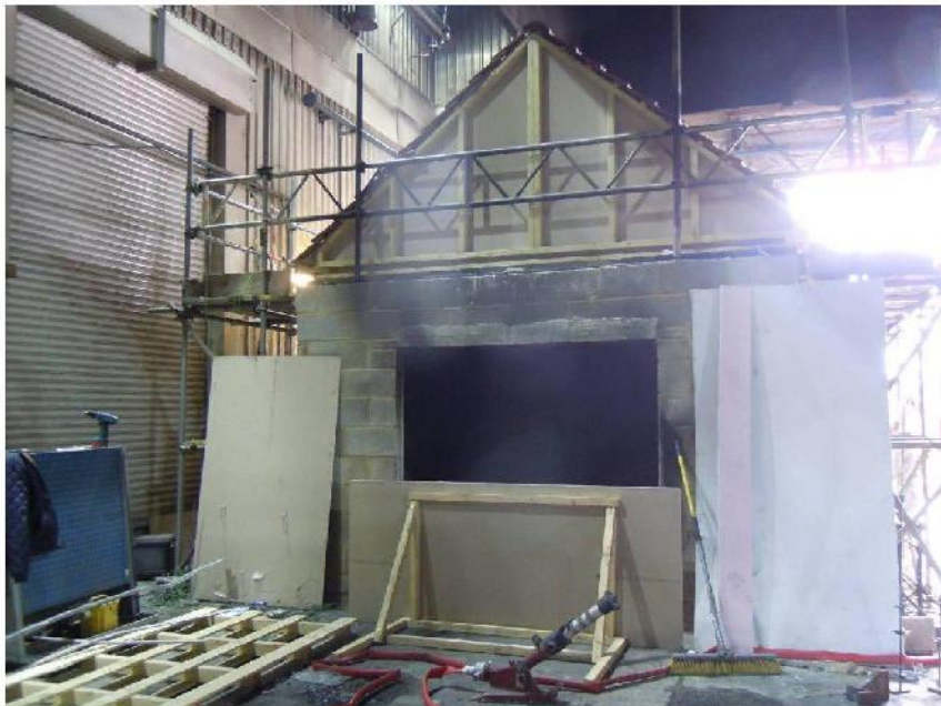
Figure 3 - (Northern) Gable end showing plasterboard to internal face of spandrel panel
