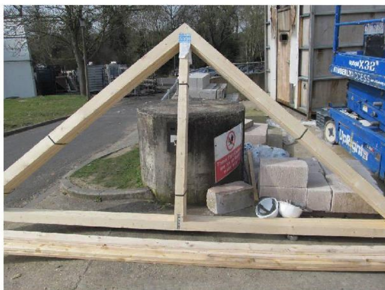
Figure 1 - Trussed rafters used for compartmentation in roof voids experiment
