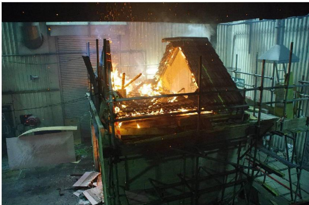
Figure 10 - Collapse of roof structure with compartmentation intact
