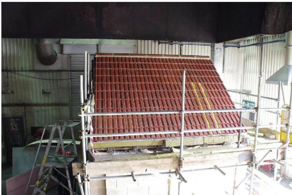
Figure 7 - Completed roof structure with spandrel panel location indicated by yellow paint
