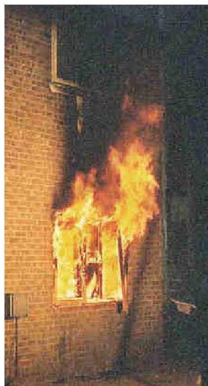
Figure 3 Fire break out from a post-flashover room on a masonry facade
