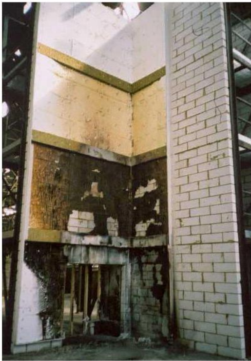
Figure 10 EPS rendered system with fire barriers after test (render removed to show damage to EPS)
