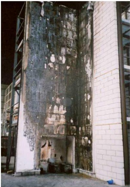
Figure 9 EPS rendered system without fire barriers after test
