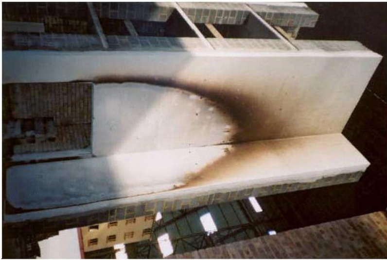
Figure 7 Limited combustible core, after test
