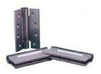
These sets of 3 self-closing hinges have adjustable closing strength functionality. Provided with intumescent backing plates they are ideal for applying to fire doors and relieve the need for additional door closers.
