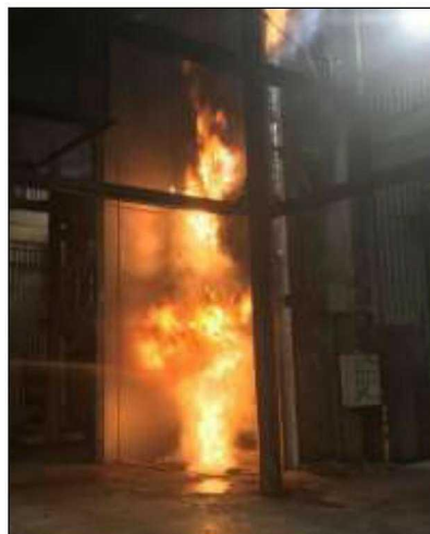
End of test in under 9 minutes: flames extend above the level of the rig
