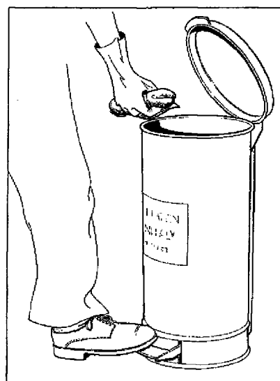
Example of metal container for cloths contaminated with flammable solvents
