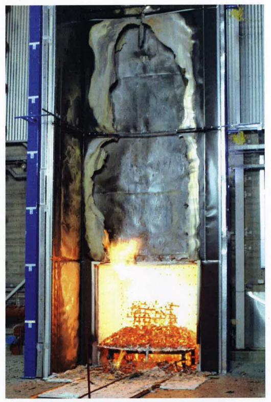
Figure C8 – Exposed face of the specimen at 30 minutes into the test
