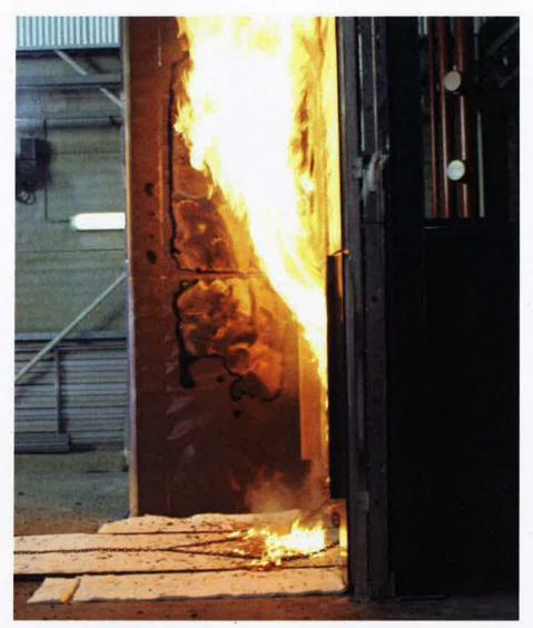
Figure C4 – Exposed face of the specimen at 7 minutes after crib ignition
