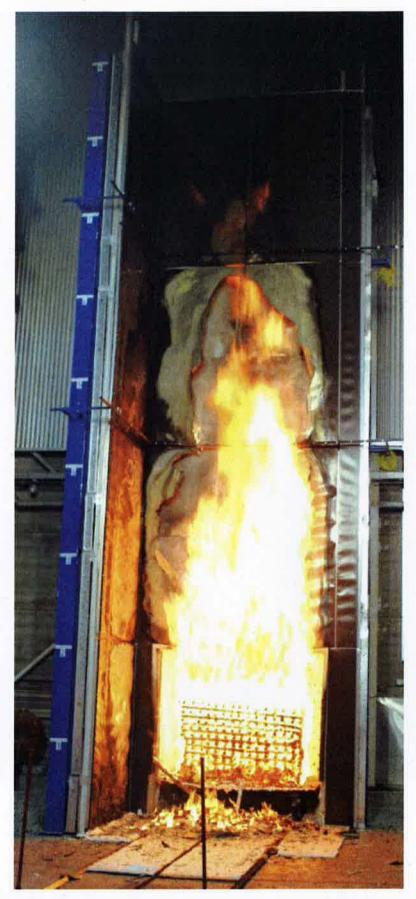
Figure C7 – Exposed face of the specimen at 19 minutes after crib ignition
