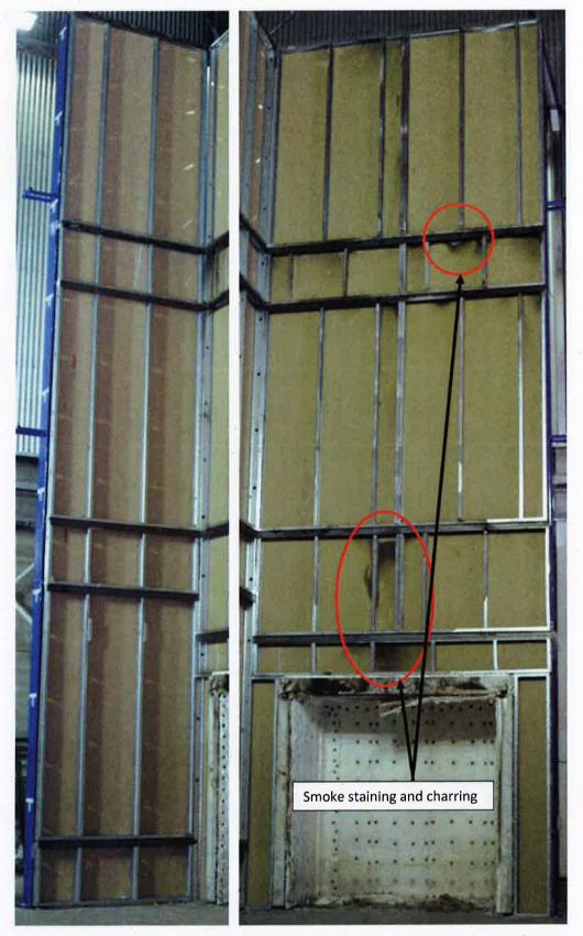
Figure D9 – Damage to the exposed side of plasterboard layer at the conclusion of testing
