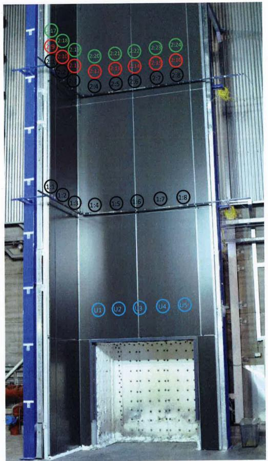
Figure B4: Thermocouple locations, elevation view
