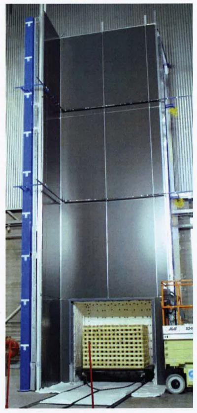
Figure C1 – Exposed face of the specimen prior to testing
