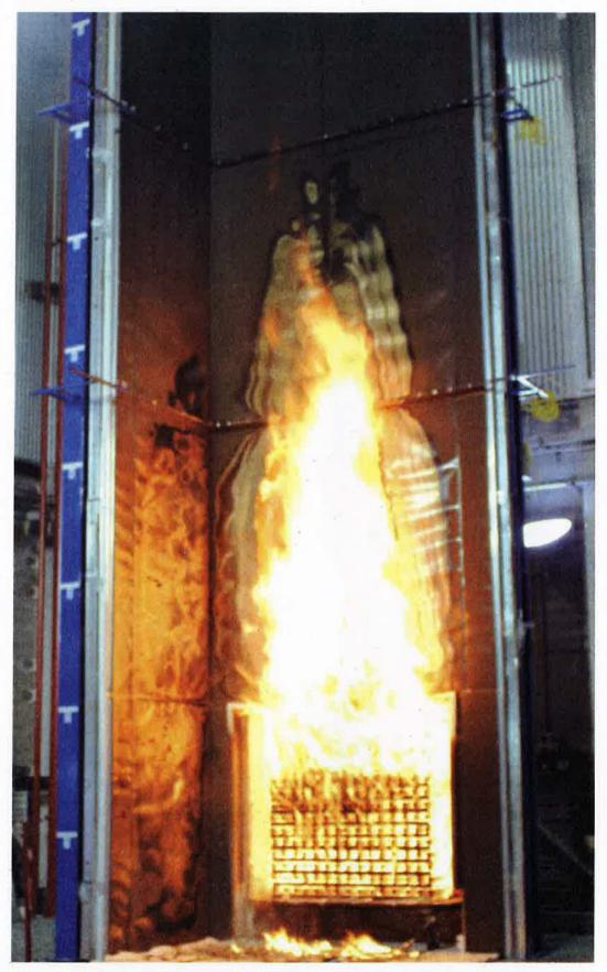
Figure C5 – Exposed face of the specimen at 11 minutes after crib ignition
