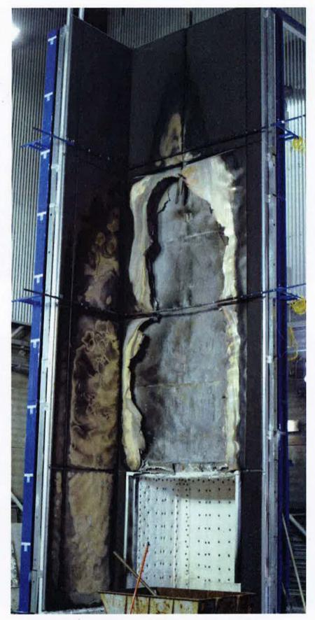
Figure C9 – Exposed face of the specimen at the conclusion of the test
