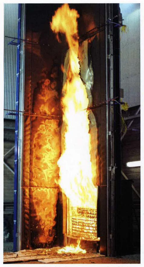
Figure C6 – Exposed face of the specimen at 17minutes after crib ignition
