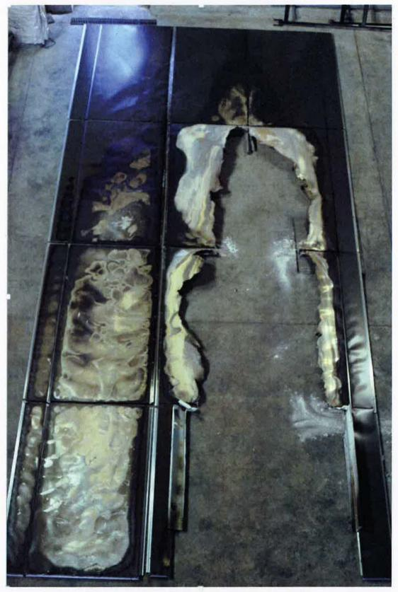
Figure D1 – Damage to the exposed aluminium skin at the conclusion of testing
