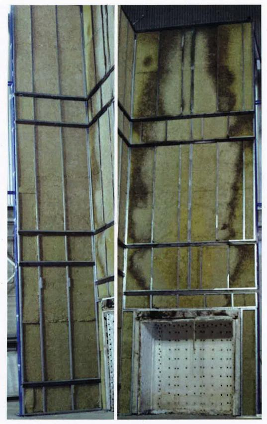
Figure D7 – Damage to the Rockwool layer at the conclusion of testing
