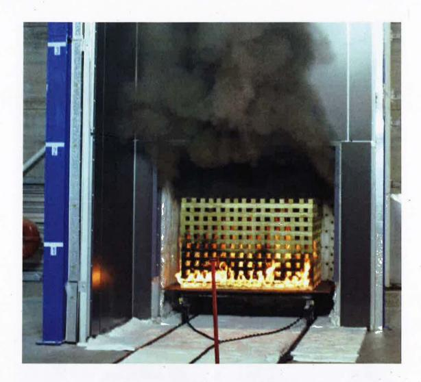
Figure C2 – Exposed face of the specimen at crib ignition
