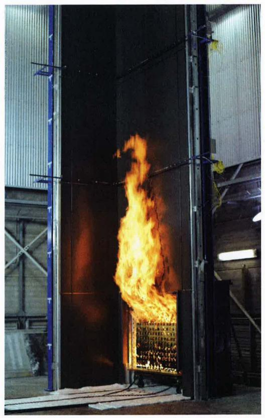
Figure C3 – Exposed face of the specimen at 3 minutes after crib ignition
