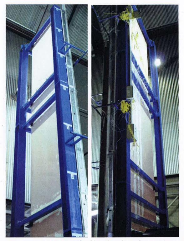
Figure C2 – Unexposed face of the specimen prior to testing
