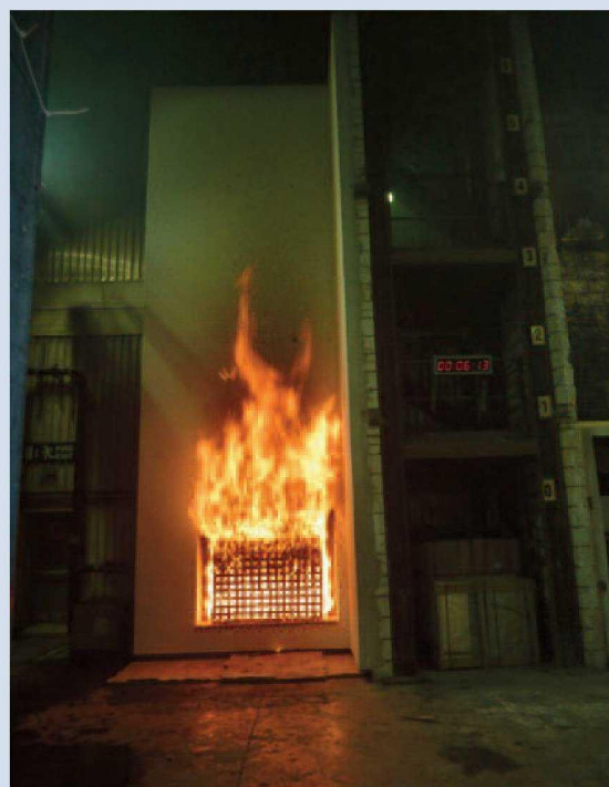
Figure 4: Kingspan Kooltherm® K5 External Wall Board being tested to BS 8414: 2002. Picture courtesy of Insuletics.
