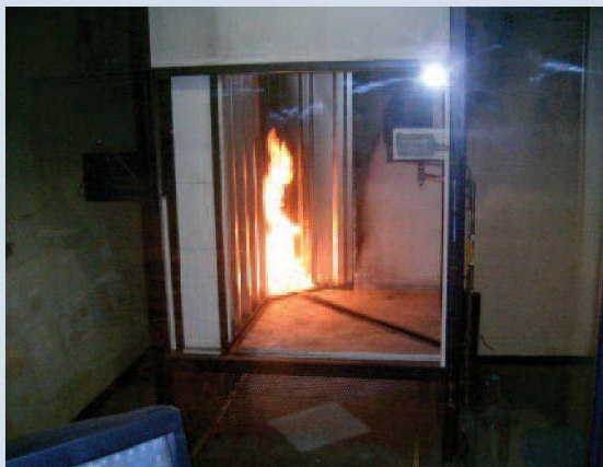
Figure 1: Kingspan Thermaroof ® TR26 LPC/FM being tested 'in application' to the Euroclass system.
