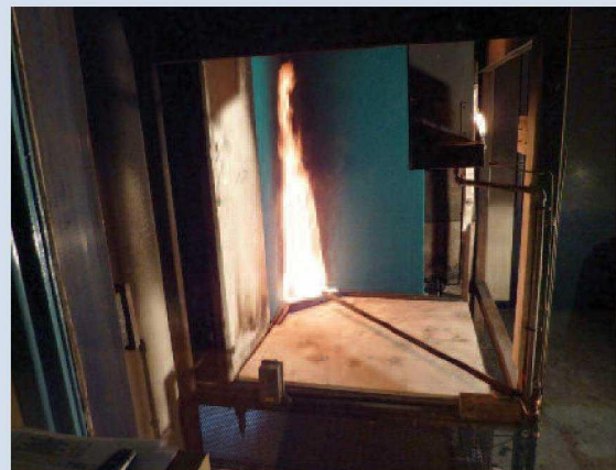
Figure 2: Kingspan Kooltherm ® K5 External Wall Board being tested 'in application' to the Euroclass system. Picture courtesy of Insuletics.
