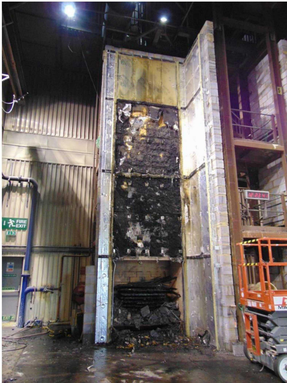
Figure 16. Full-height photograph of system following removal of ACM panels and aluminium rail substructure.
