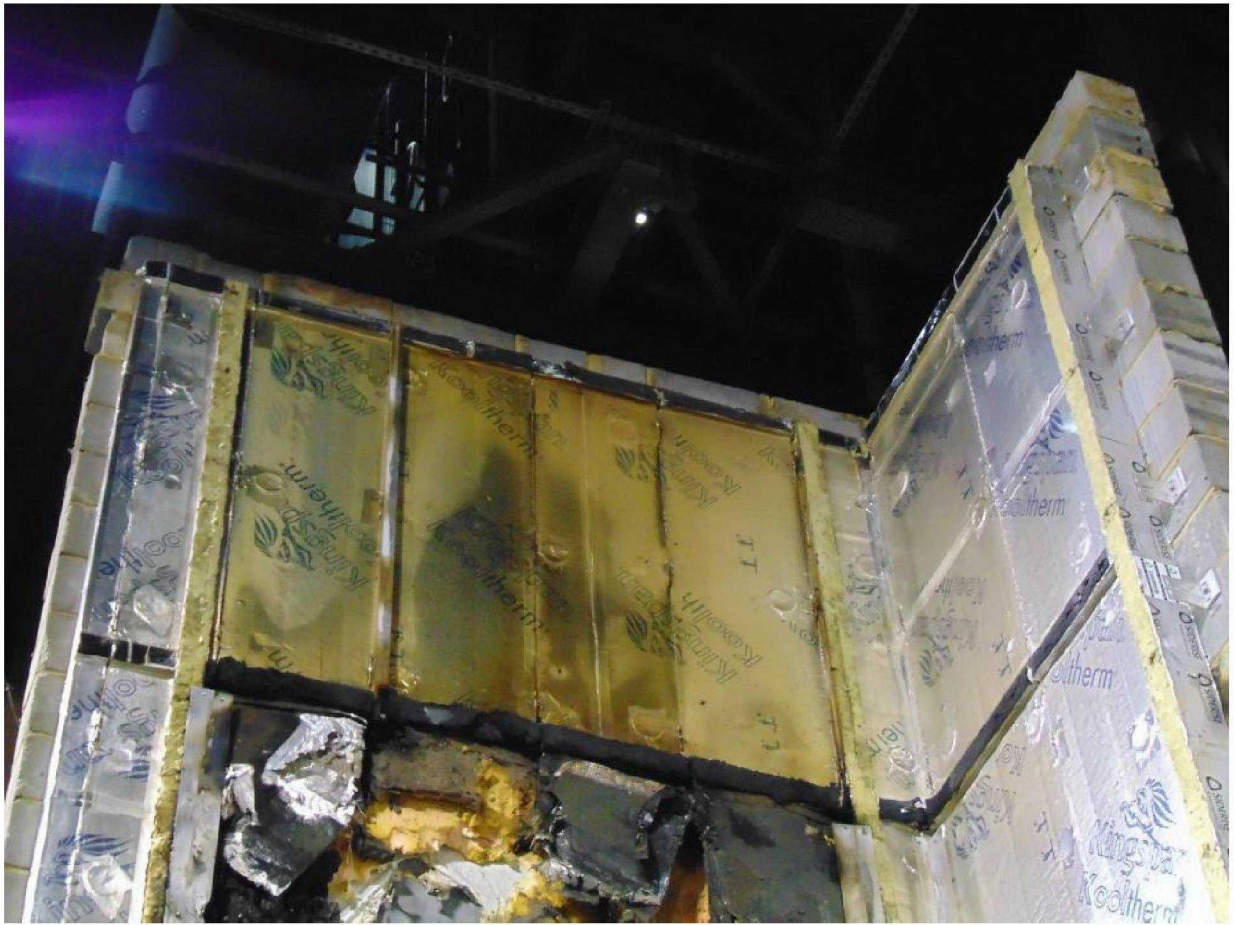
Figure 19. Post-test photo between third and fourth row Siderise RH25G 90/30 horizontal open state cavity barriers.
