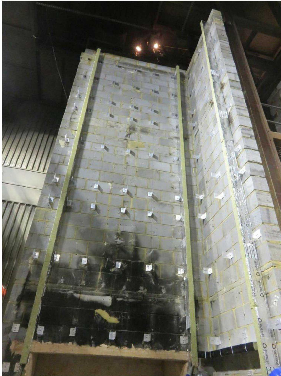
Figure 4. 'L'-shaped aluminium brackets installed with Siderise RSV 90/30 vertical cavity barriers fitted on main and wing wall.
