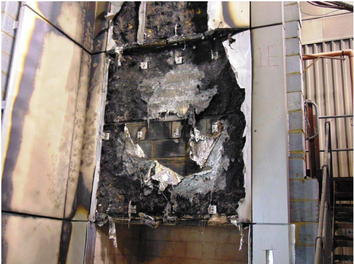
Figure 17. Row 1 post-test (main and wing wall, approximately 2300mm above combustion chamber).
