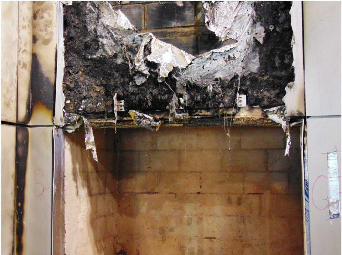
Figure 16. Row 0 post-test (combustion chamber, main and wing wall).
