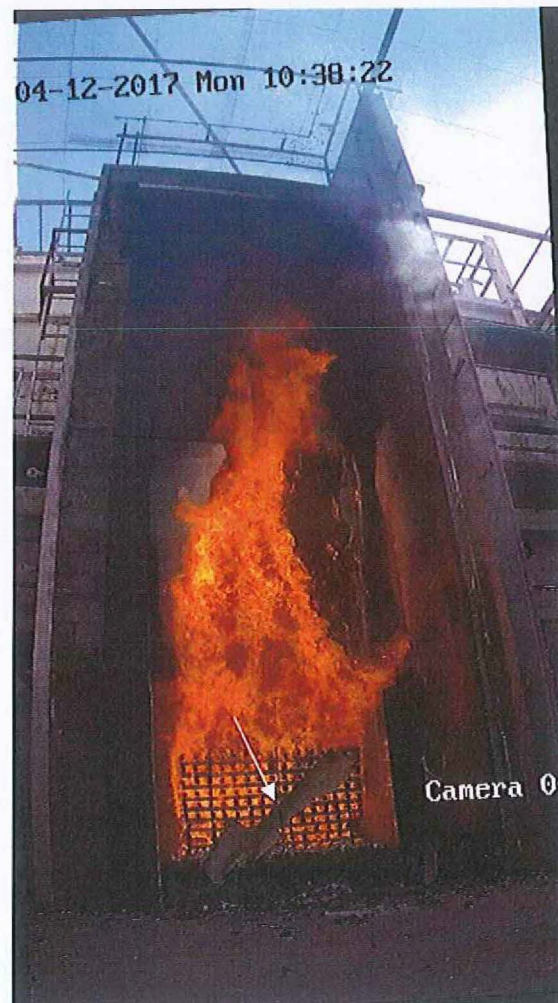
DLP C2753B/0004 Panel M5 fell from the main wall.
