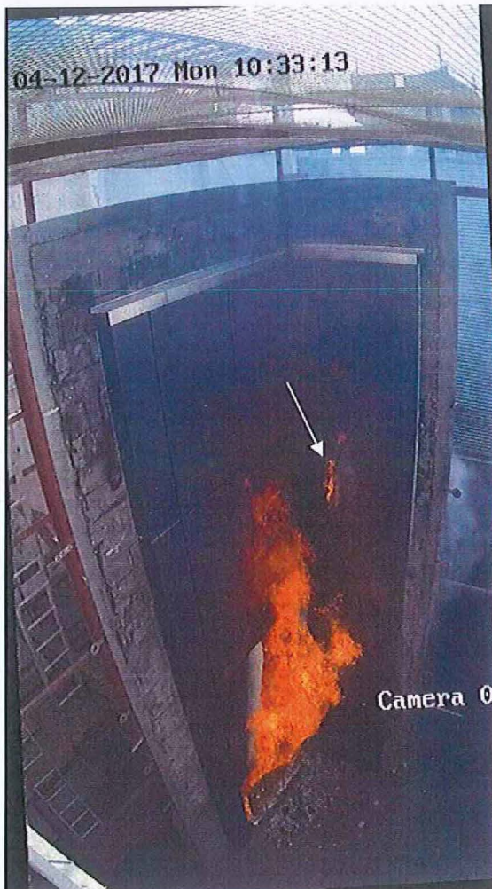
DLP C2753B/0003 Continuous flame observed on W5 & W6 vertical joint.
