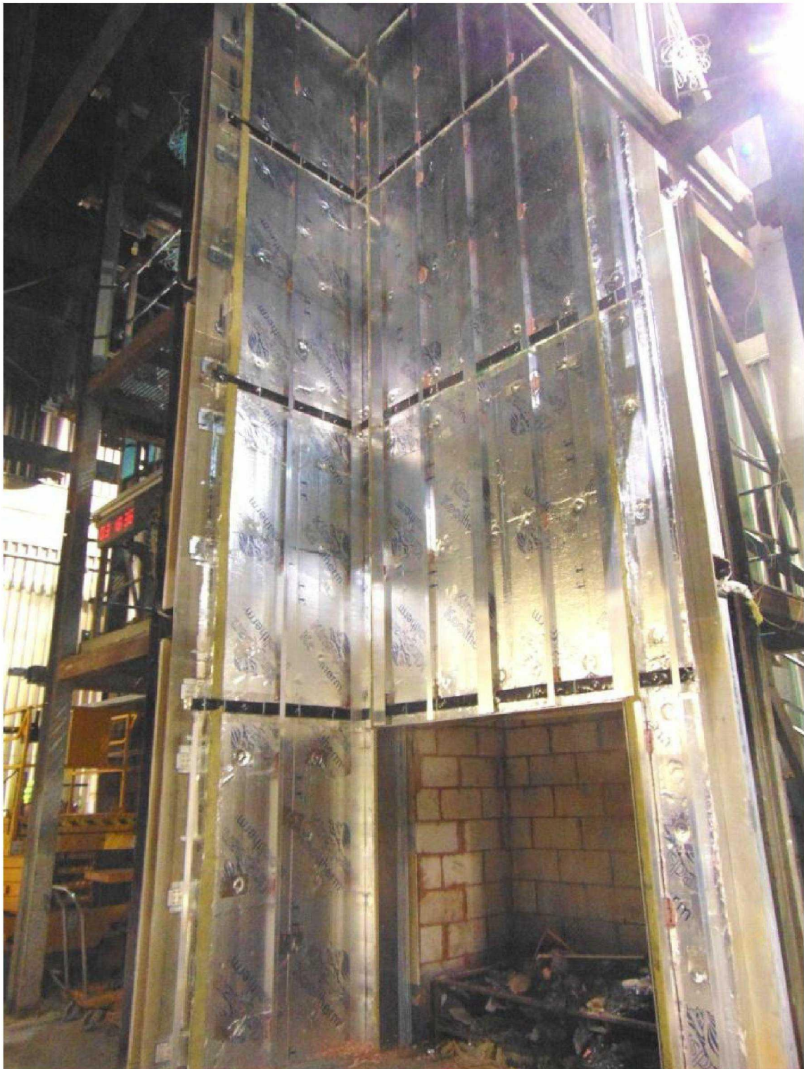
Figure 8. Vertical rails fitted to system.
