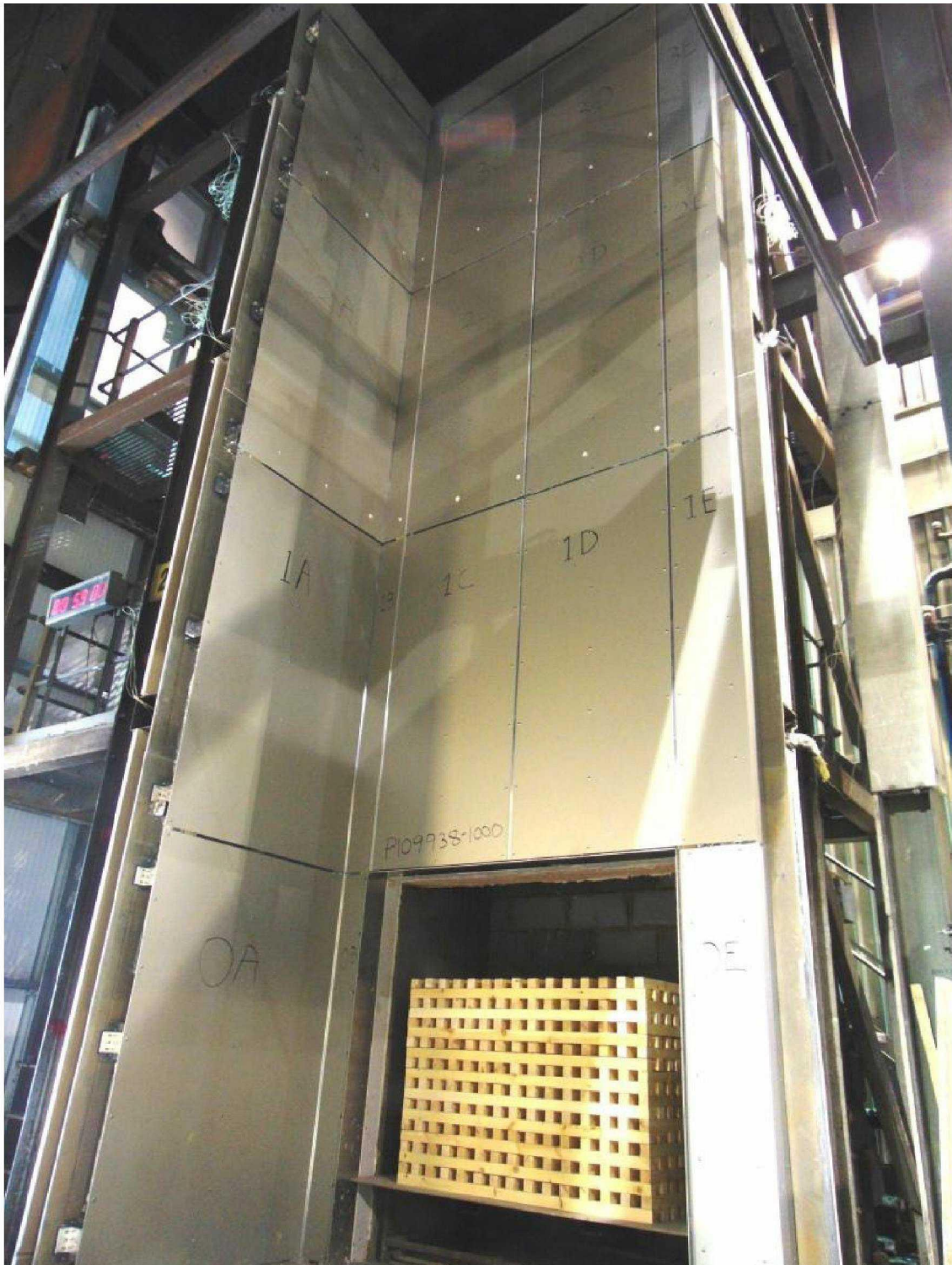
Figure 9. Full-height photograph of cladding system prior to test.
