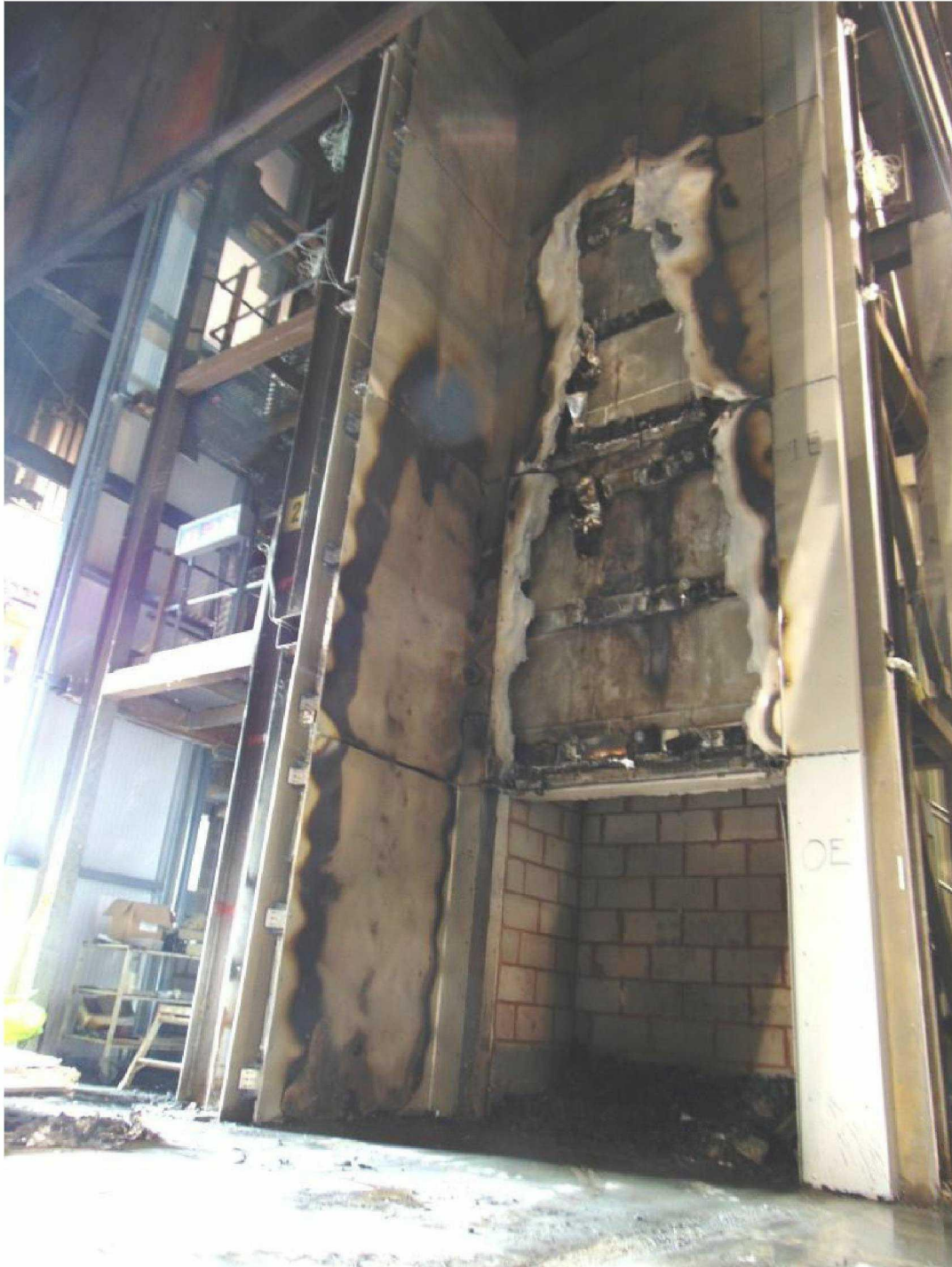
Figure 20. Full-height photograph of cladding system immediately after test.
