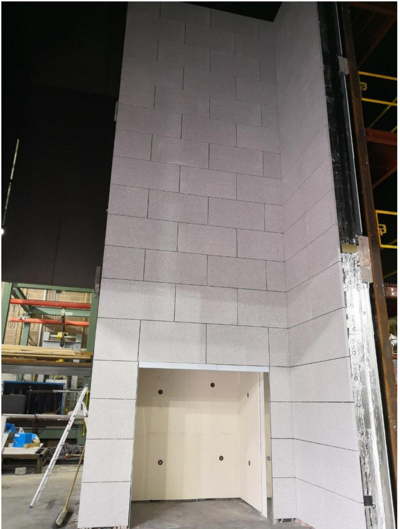
Figure 4.8. Cladding system before test.
