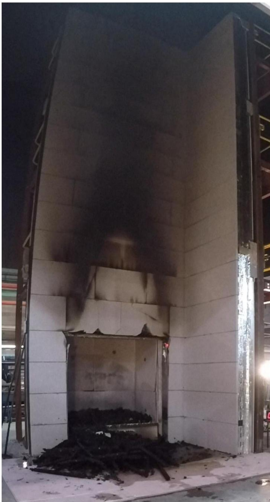
Figure 4.15. Cladding system just after the fire test (60 min 01 sec after ignition of the crib).
