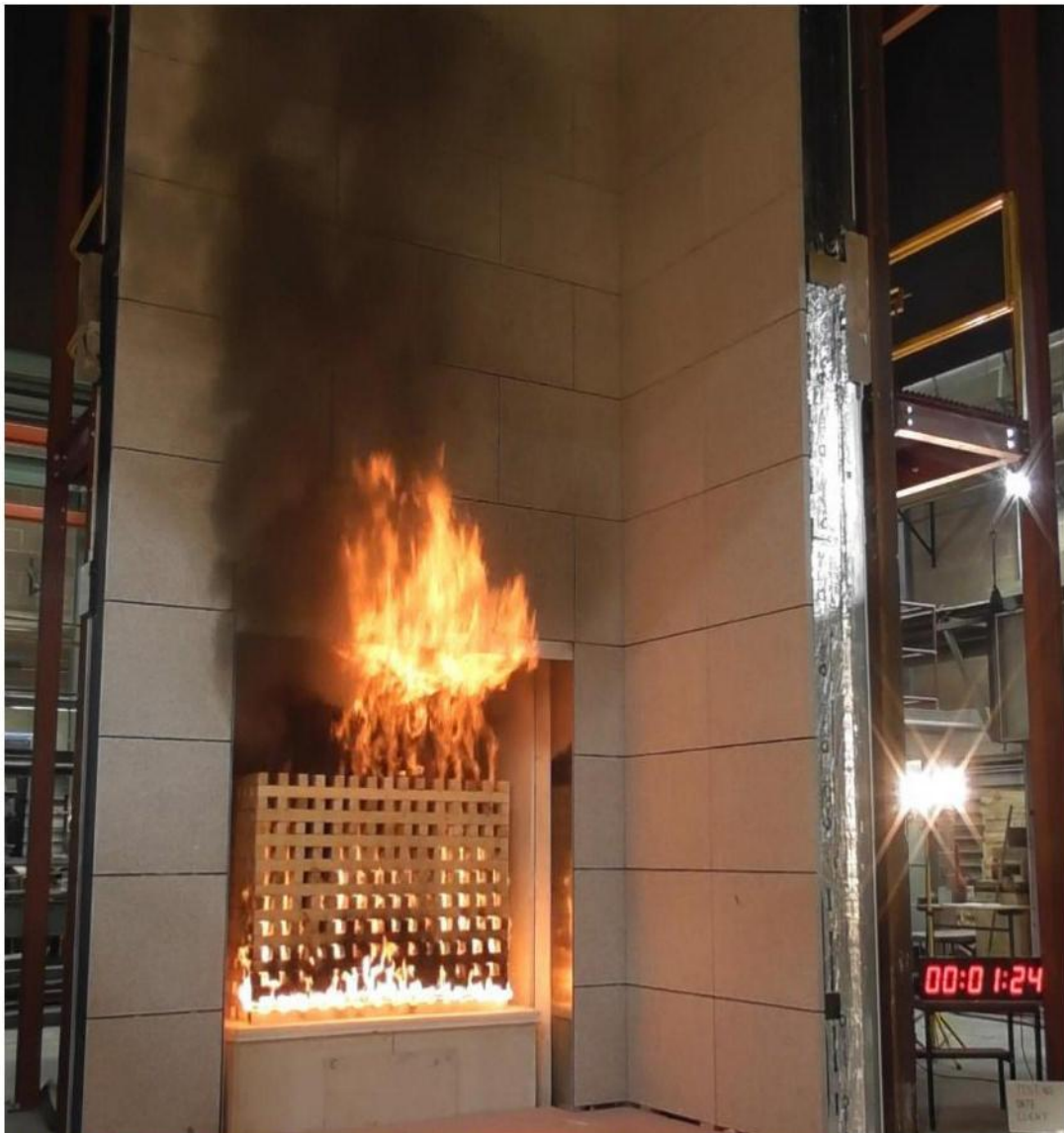
Figure 4.11. Cladding system during the fire test at start time t_s (01 min 24 sec after ignition of crib).
