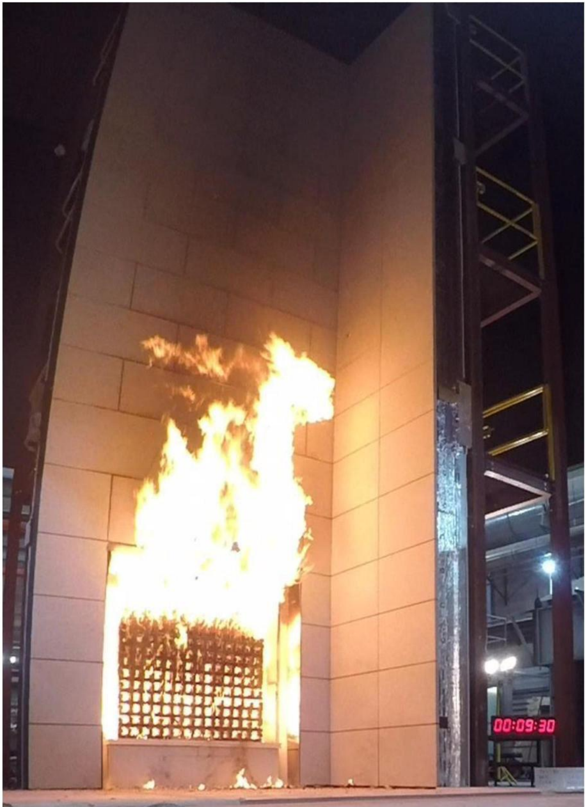
Figure 4.12. Cladding system during fire test (09 min 30 sec after ignition of the crib).
