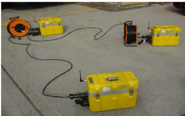
Figure 3 – TSR2000 connected in series mode
