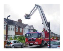
The Brigade has 11 frontline aerial appliances – four turntable ladders (TL) located centrally and seven aerial ladder platforms (ALP) located around the perimeter of the Brigade. There are two versions of the ALP, the 320 and 325 and a number of hydraulic platforms (HP) are still available as spares.
