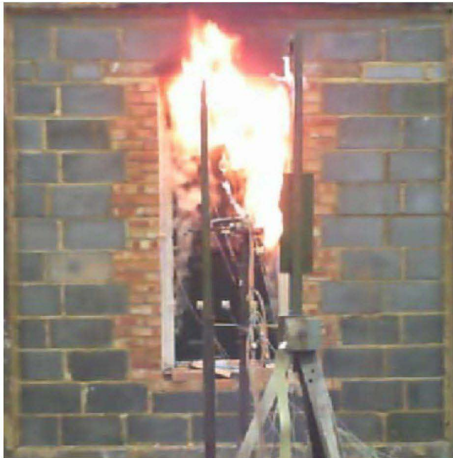
Unexposed face of specimen at end of test (28 minutes).
