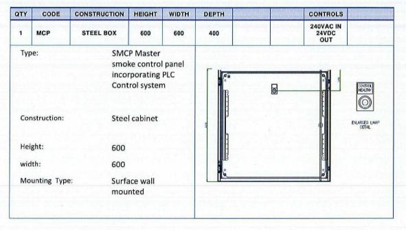
The master smoke control panel will be a steel wall mounted unit. The dimension of the panel will be 600mm High x 600mm Wide x 400 Deep with full PLC driven control system. The panel will be wall mounted in the electrical riser on the first floor.
