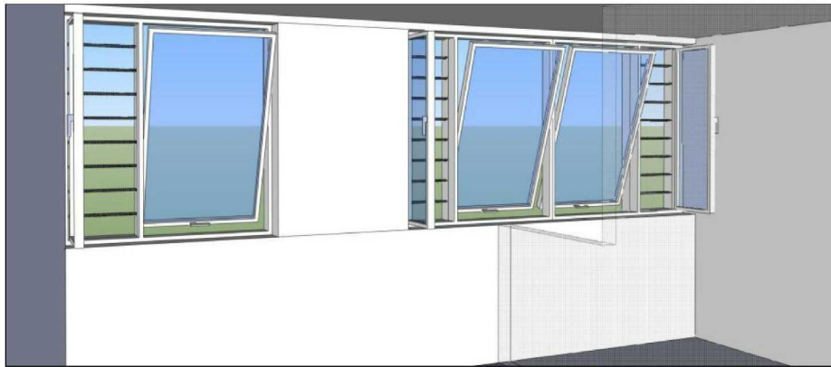
Figure 4-5 Safe purge ventilation
