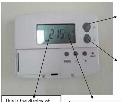
This is the button to press to turn up the temperature of your heating
