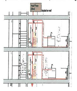
Option B2 - Gas Fired Heat Pump with Central Storage
