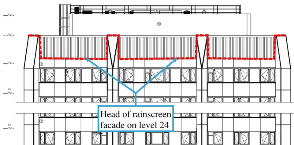
Figure F.3 Elevation of Grenfell tower- Top of external wall cavity indicated with red dashed line
