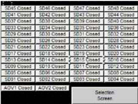
Figure J.61: Fireman’s override damper status screen taken from MET00018074.z2g using WindOI-NV2.
