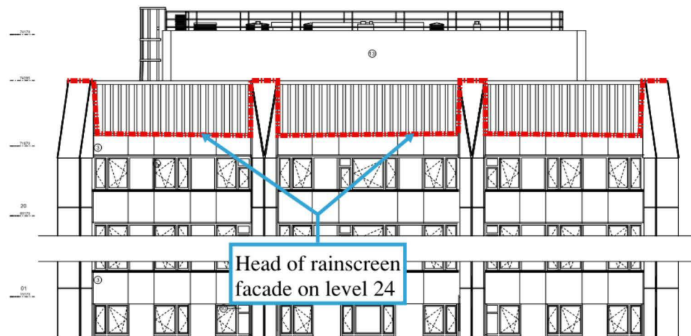
Figure 11.32 Location of the head of the rainscreen cladding at level 24 (adapted from drawing 1265 PL 322 Rev 03, RYD00092648)
