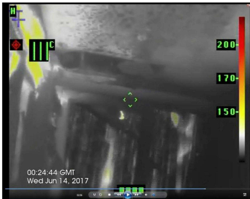
Figure 13.2: Thermal image of kitchen window. MPS description: “kitchen window failed and molten dropped down outside” at 01:21 [time adjusted] on 14 June 2017 (MET00006109)
