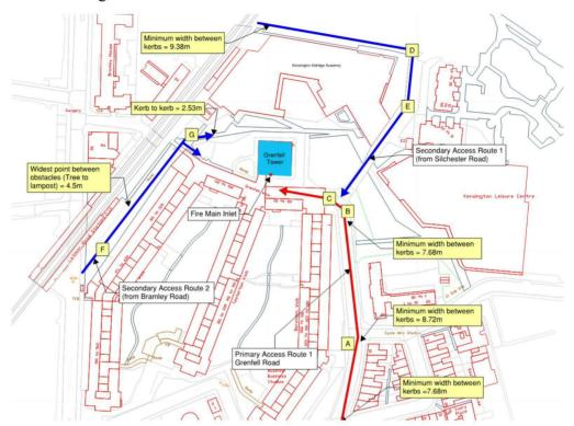
Figure 17.38: Primary vehicle access route to Grenfell Tower and secondary access routes to the other elevations, summary of onsite measurements of 7th November 2017
