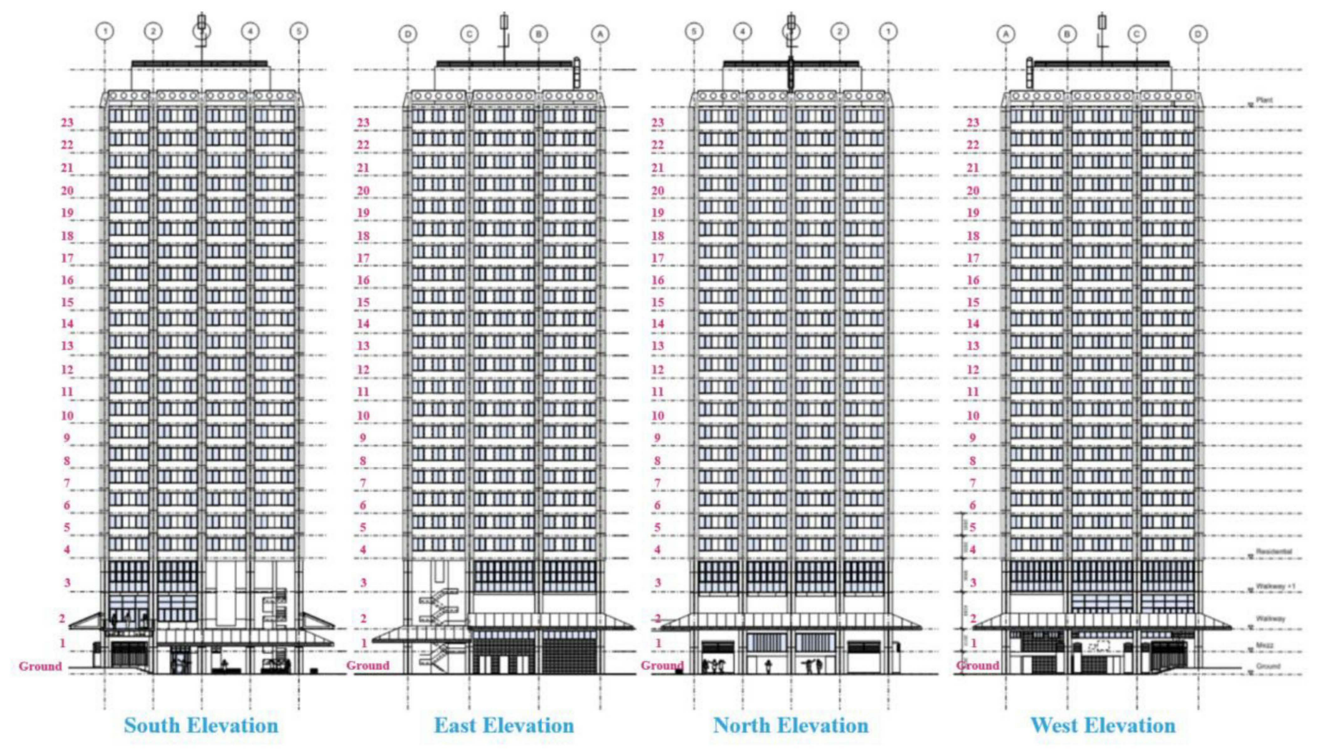
Figure 4.14: Original construction of Grenfell Tower – building elevations (CCL00000028)
