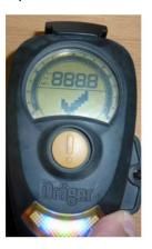
30. Following this sequence – 'Switch-Off' the unit by pressing and holding the left button
