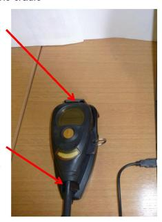
8. Switch the BG 7000 unit on by pressing the Left button
