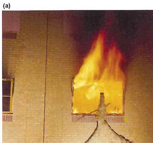
Figure 4: (a) Fire breakout from a post-flashover room on a masonry facade, (b) result of the flashover
